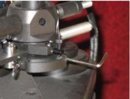
Fig.12 Removing horizontal trough
