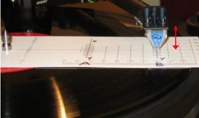
Fig. 15 Alignment at B
