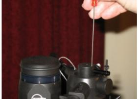
Fig.10 Fixing vertical damping holder
