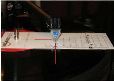
Fig. 14 Alignment at A
