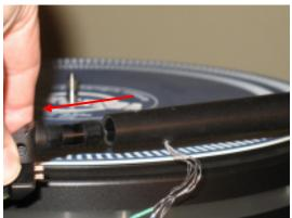
Fig.7 Removing headshell
