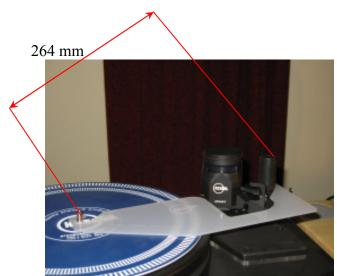
Fig.3 Protractor for pivot to spindle distance
