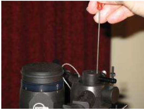
Fig.10 Fixing vertical damping holder
