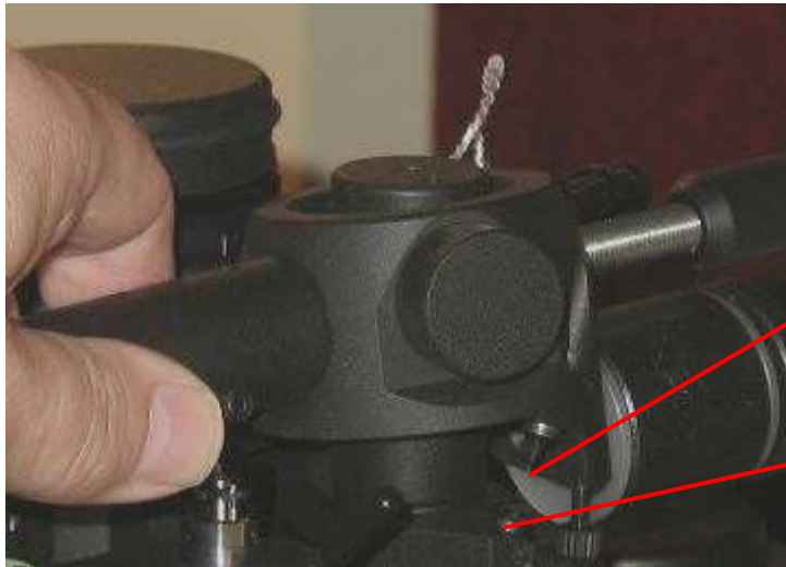
Fig.4 Assembling the tube onto the horizontal bearing tower.
