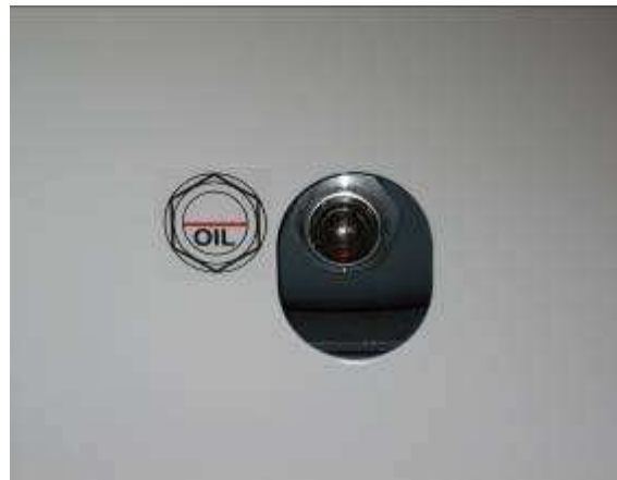
Compressor oil level in bubble
