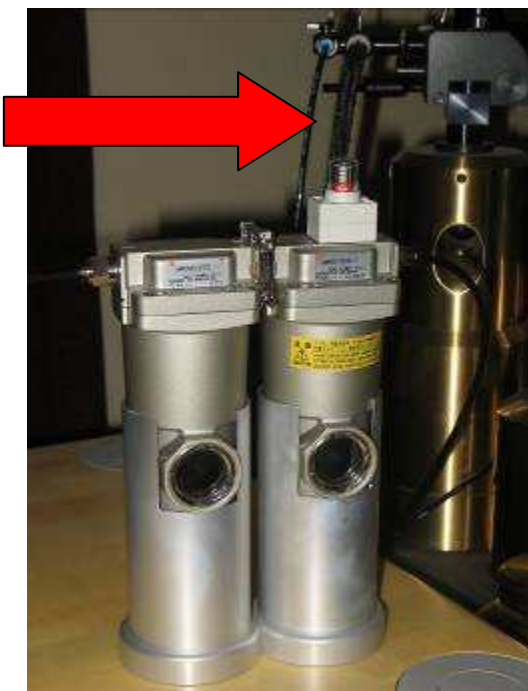
Silver filters-dryers- see arrow for airflow
