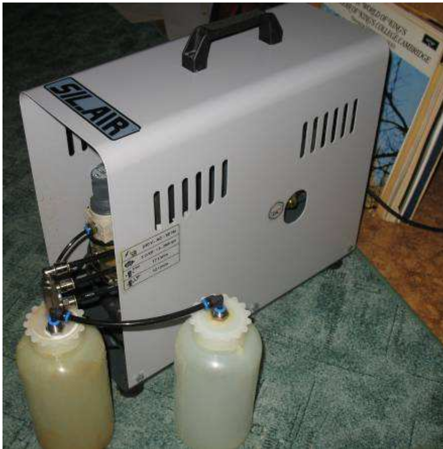
Compressor with “double drain bottle system.”
