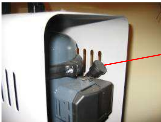
Compressor - rear view - air intake filter
