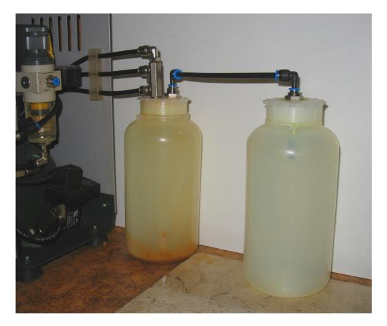
Air Line compressor- Double drain bottle since 2009 as standard
