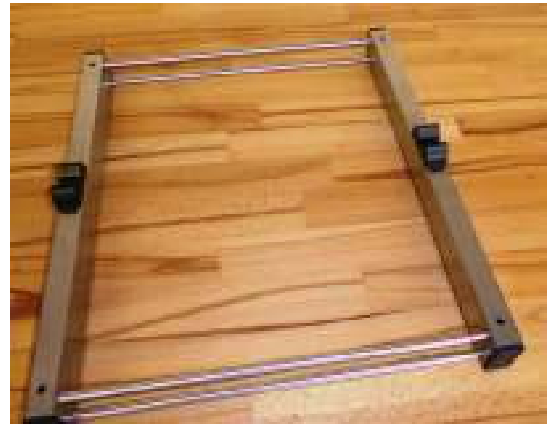
Fig. 2.3. Frame with 4 rods nearly assembled
