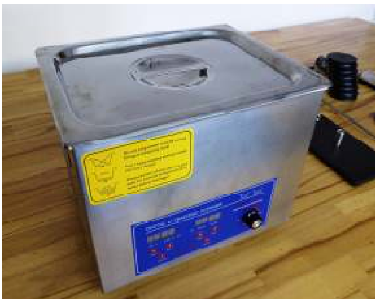
Ultrasonic cleaner bath- typical sample
