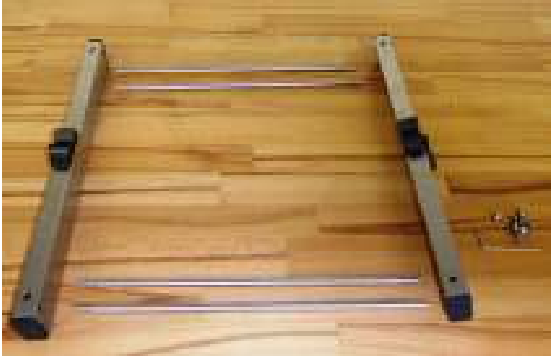
Fig. 2.1. Frame parts: 2 square tubes with 4 rods
