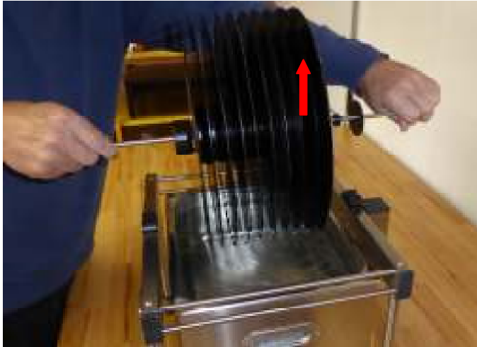
Fig. 10.0. Lifting spindle with LPs out of bath.
