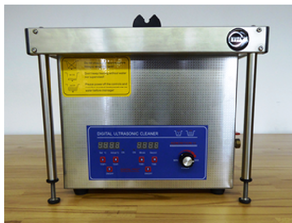
Fig.4.3. Level frame with US cleaner bath
