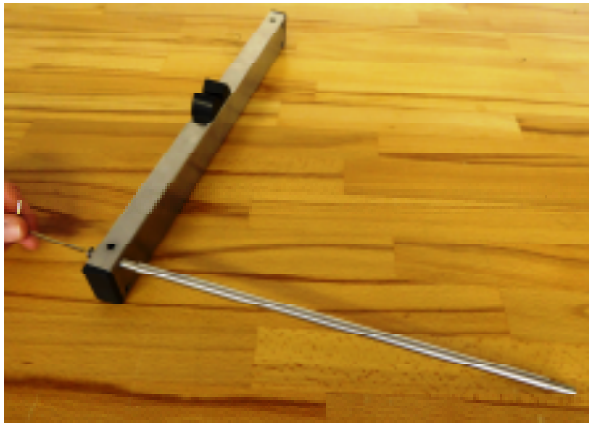
Fig. 2.2. Fixing rod into square tube
