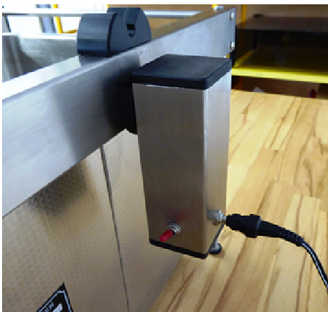
Fig. 5.0. Motor, switch, plug in DC supply
