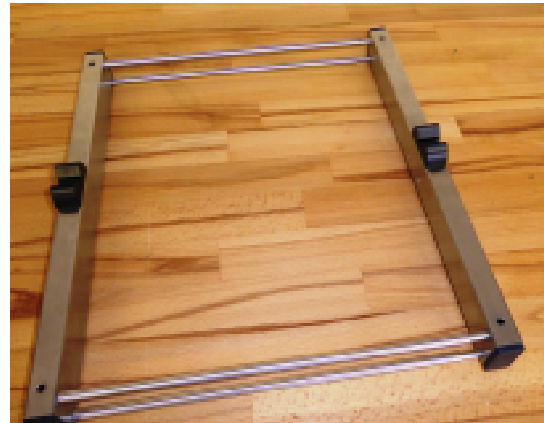
Fig. 2.3. Frame with 4 rods nearly assembled
