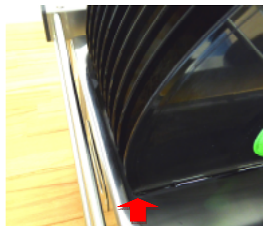
Fig. 9.5. Gap between edge of bath and LPs
