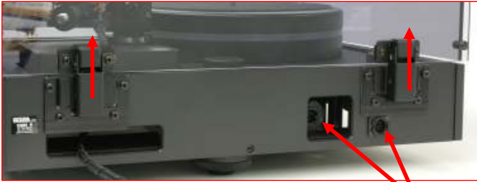
Fig. 5 Rear panel ( hinges & XLR connections)
