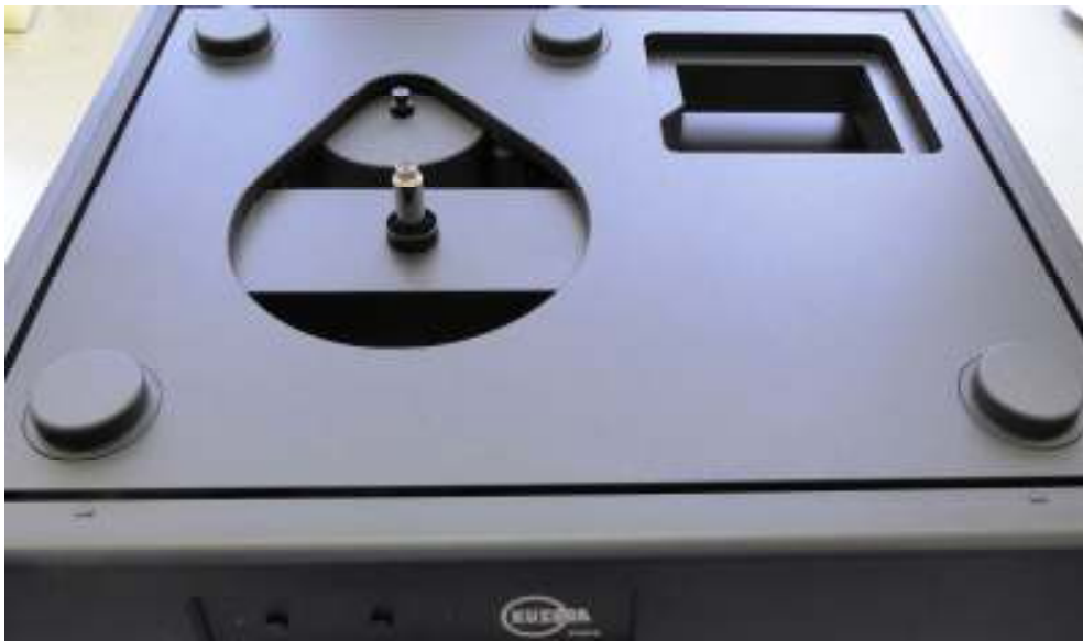
Fig. 3. Top plate in the outer frame with 4 height knob adjustments
