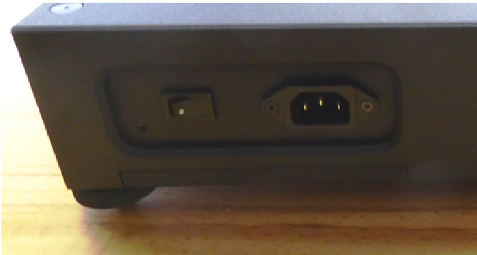
Fig. 7. Rear panel with mains switch
