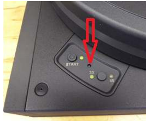
Fig. 8A. Two green LED showing 33 rpm
