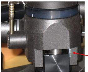
Fig. 2.VTA tower side-rough scale
