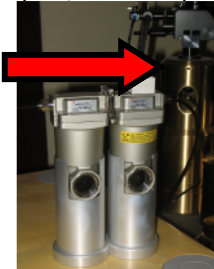
Fig. 11. Silver filters- see arrow for airflow
