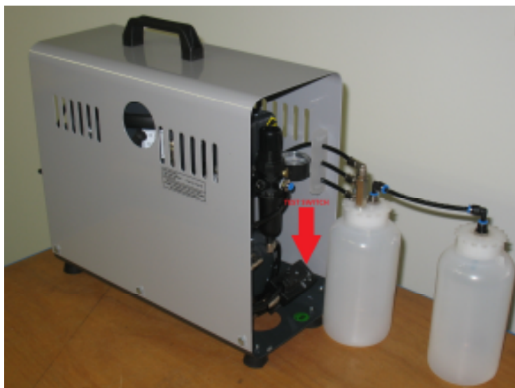
Fig. 7. Compressor with Double PVC drain bottles
