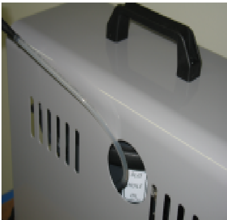
Fig. 9. Oil filling from side of the compressor
