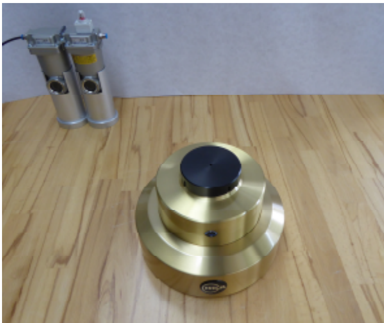
Fig. 6. Base with air bearing-for now ignore silver filters
