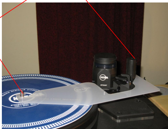
Fig.3 Protractor for pivot to spindle distance
