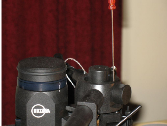
Fig.11 Removing vertical trough
