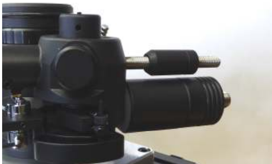
Fig. 9. Full counterweight complement
