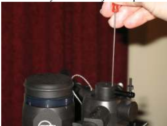
Fig.12. Fixing vertical damping holder
