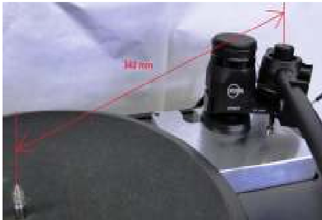
Fig.4. Distance for pivot to spindle
