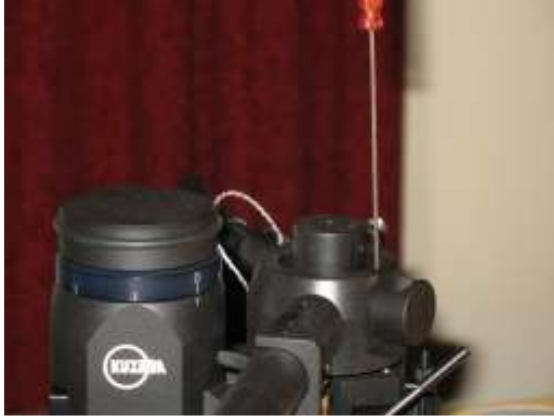
Fig.13 Removing vertical trough
