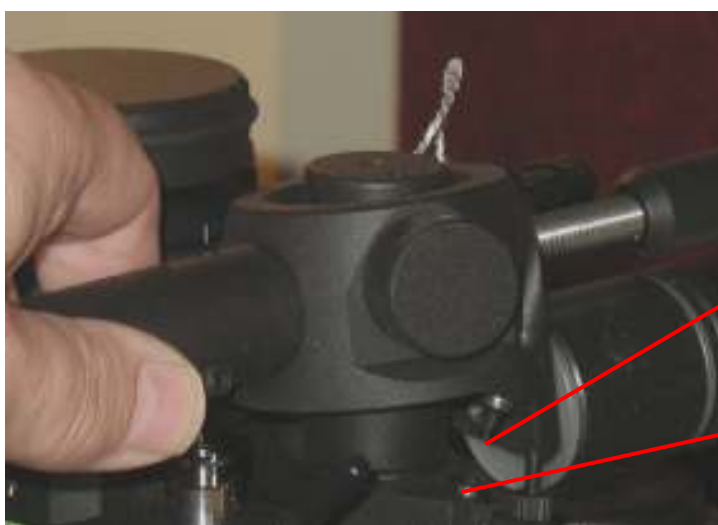
Fig.6. Assembling the tube onto the horizontal bearing tower.
