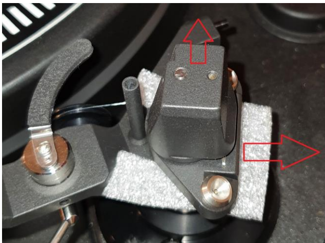
Fig. 6. Arm tower-removing transport foam
