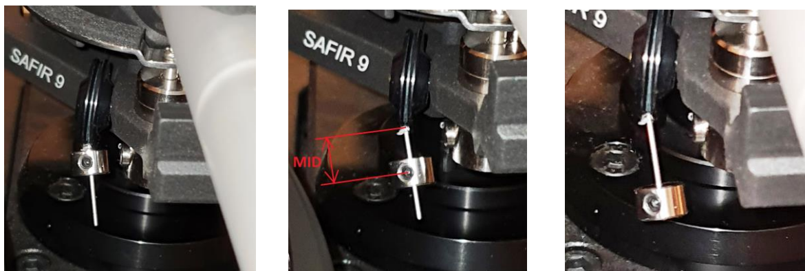
Fig. 15. Bias adjustment distance: minimum-middle-maximum
