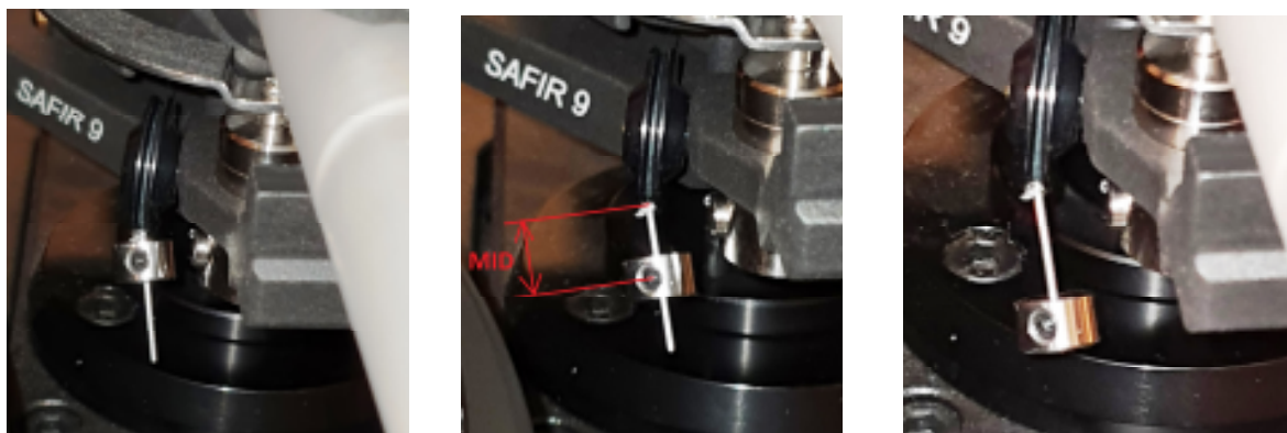
Fig. 15. Bias adjustment distance: minimum-middle-maximum
