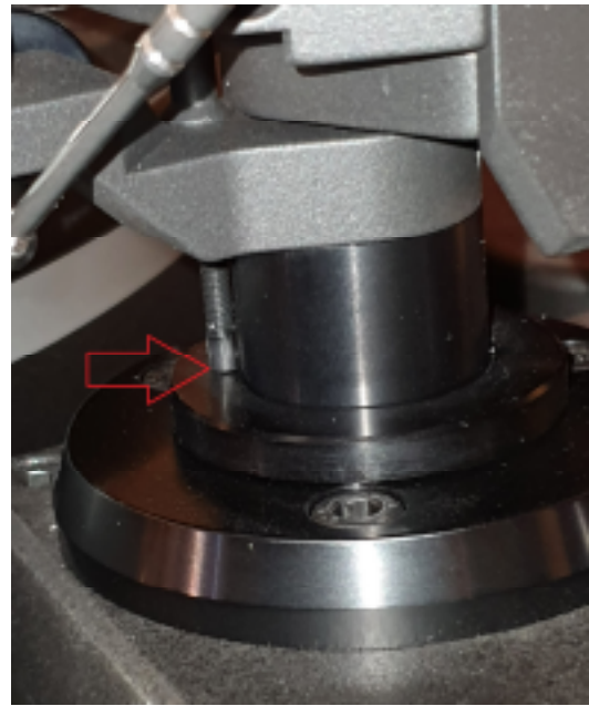
Fig. 13a. VTA screw on VTA height ring-5mm
