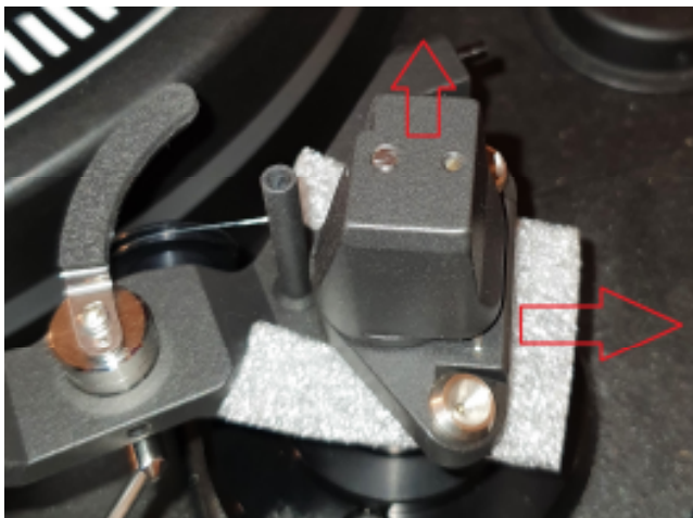
Fig. 6. Arm tower-removing transport foam
