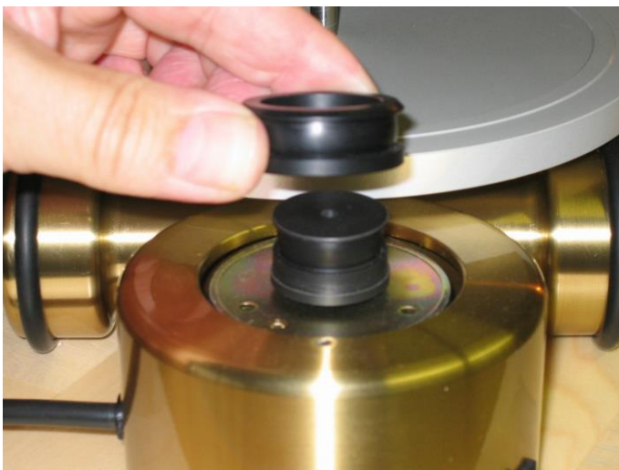
Fig. 8 45 rpm crown ring adaptor ( no PS)
