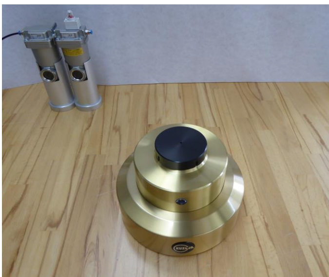
Fig. 2. Base with air bearing-for now ignore silver filters
