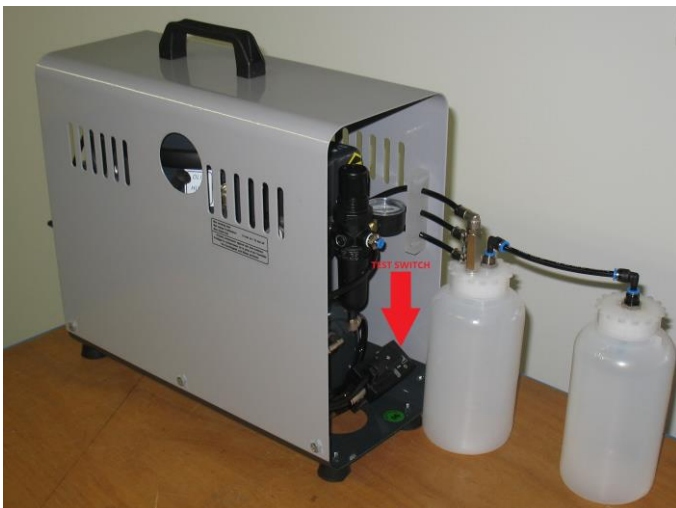
Fig. 3. Compressor with “Double PVC drain bottles”
