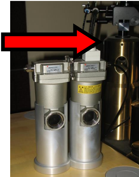
Fig. 7. Silver filters- see arrow for airflow
