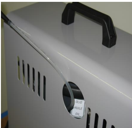
Fig.5. Oil filling from side of the compressor
