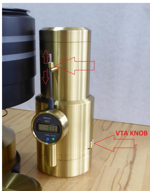
Fig. 23. Tonearm tower raised with support pad
