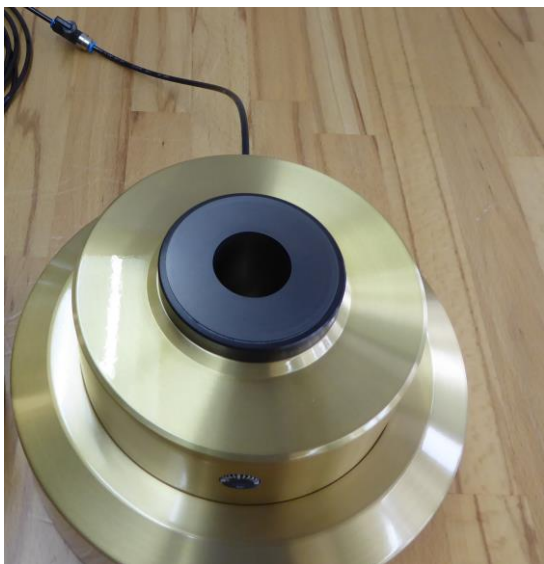
Fig. 10. Base with airbearing
