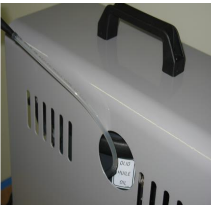
Fig.5. Oil filling from side of the compressor
