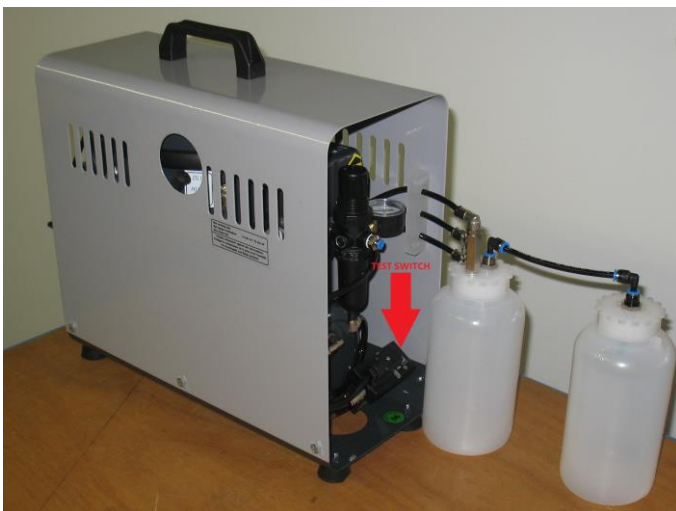
Fig. 3. Compressor with “Double PVC drain bottles”
