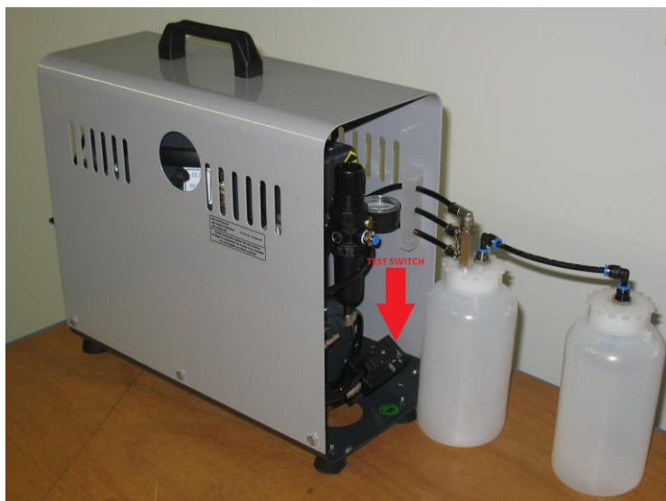
Fig. 7. Compressor with Double PVC drain bottles
