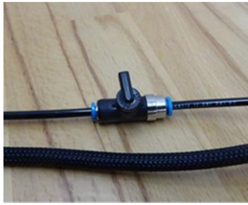
Fig. 13. Valve in closed position
