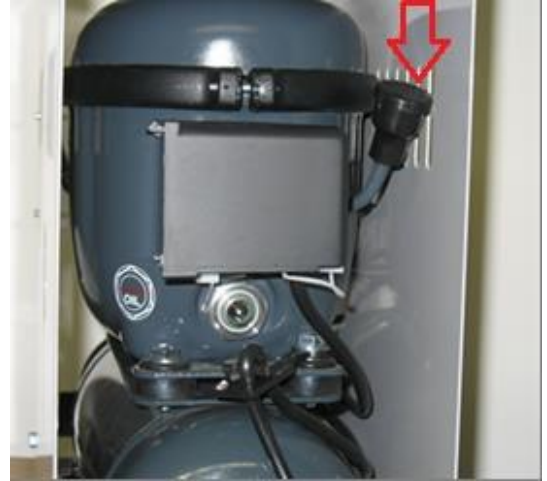
Fig. 8.a. Compressor-rear-manual fitted air intake filter
