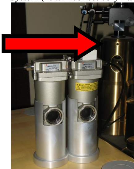
Fig. 11. Silver filters- see arrow for airflow
