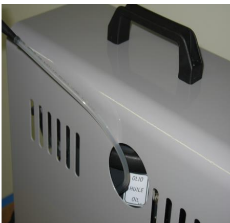
Fig. 9. Oil filling from side of the compressor
